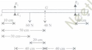
AB is the rod.  $K_1$  and  $K_2$  are the two knife edges.
